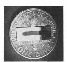
HUMIDITY SENSING ELE-MENT, developed by C. M. Stover, is shown against a background of a U.S. dime. The tiny device, made from aluminum foil with a thin anodized oxide coating, possesses extreme sensitivity and responds rapidly to humidity changes.
